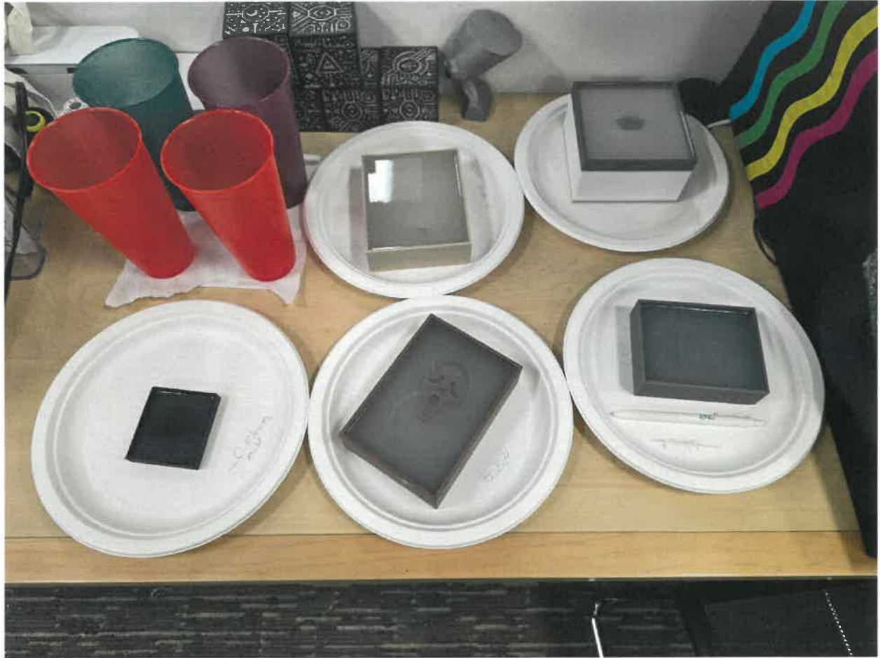
Silicon molds made from 3D designed and printed parts
